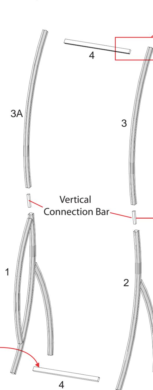
NOTE: When assembling horizontals they should be placed approximately one inch from TOP and BOTTOM.
