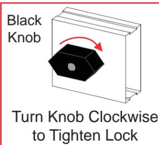
Turn Knob Clockwise to Tighten Lock
