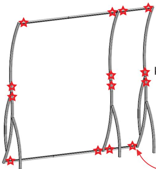
STAR indicates location of knobs on BACKSIDE of unit.
